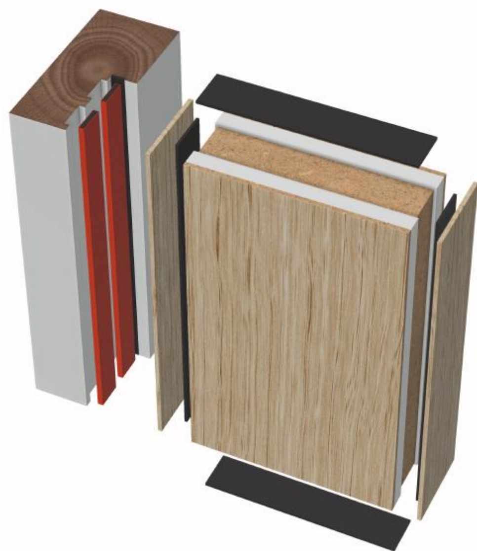
(A): Timber framed single door intumescent seal arrangement
